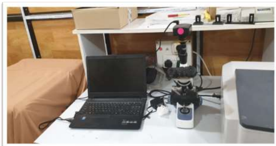
Figure (4) : A picture showing the light microscope used to photograph samples with magnification (10x).
